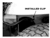
**IMPORTANT:** Do not kink hoses exiting the power unit. Leave enough excess for a generous bend in the supply lines when assembling clip to tractor.
